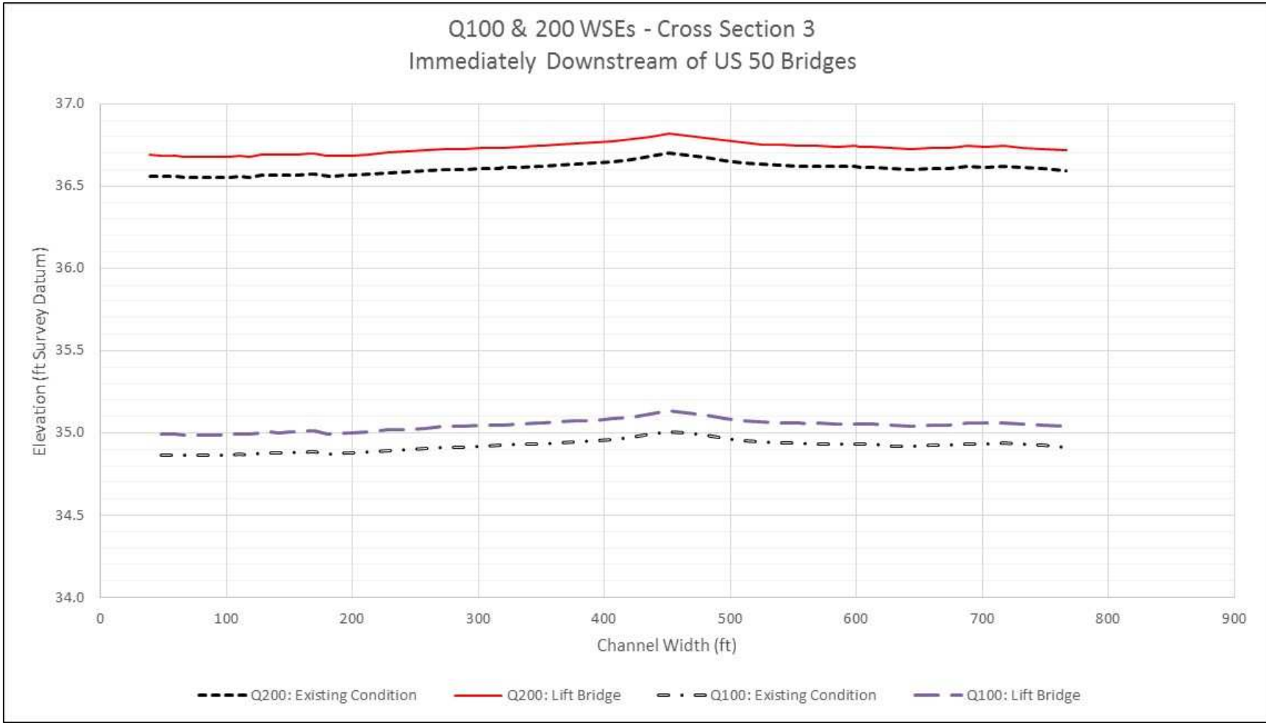
Figure 13. Cross Section 3, exaggerated scale to show WSE difference
