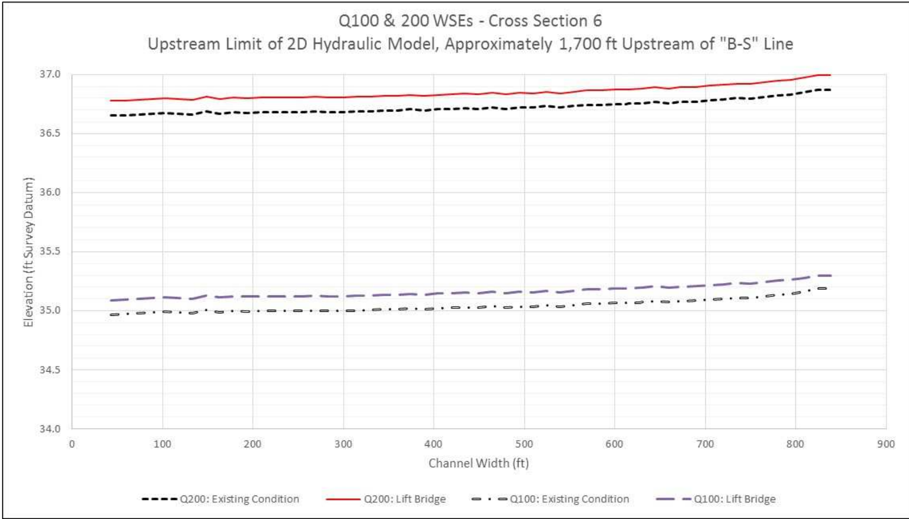
Figure 16. Cross Section 6, exaggerated scale to show WSE difference
