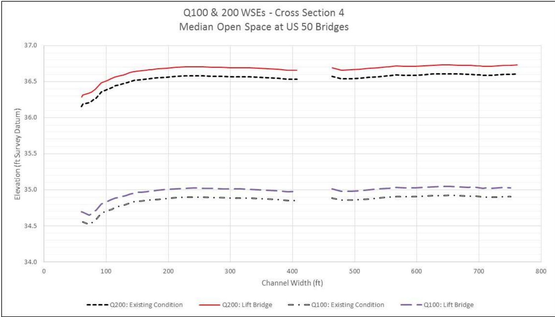
Figure 14. Cross Section 4, exaggerated scale to show WSE difference
